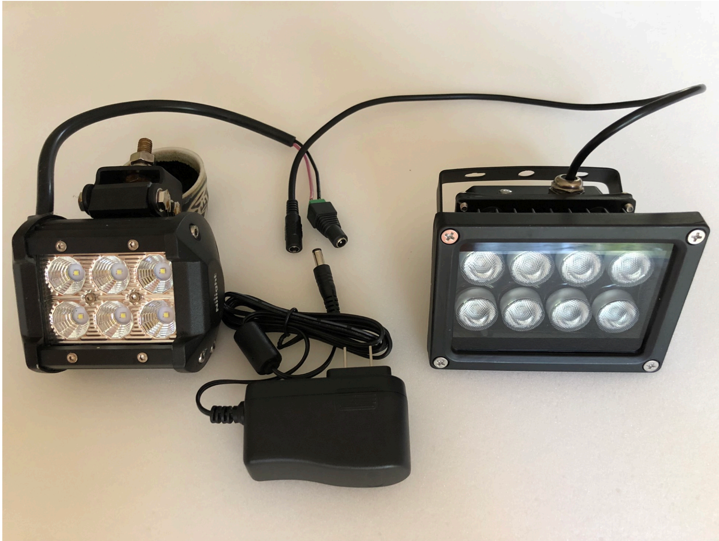
White floodlight (18W), 12V power cube, Infrared floodlight (8W)
