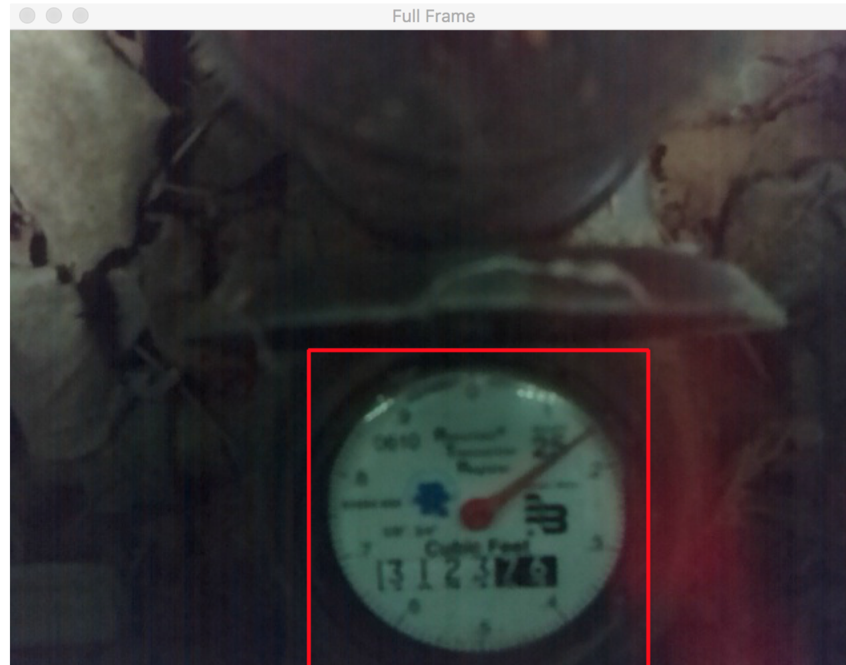
Full Frame from RPi PiCamera. Lit with 24 low power LEDs to minimize reflections and glare
